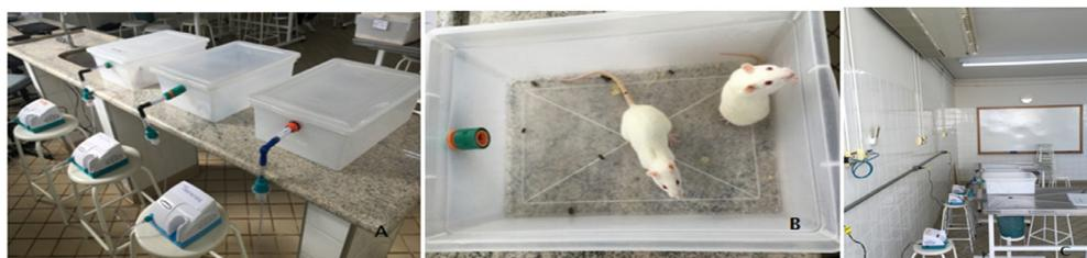
**Figure 2.** Nebulizer system developed by the students of Centro Universitário Barão de Mauá for animal experimentation. A: Adaptation of plastic boxes with inhalers identified with the group of animals to be placed; B: Accommodation of the animals; C: Climatization.
